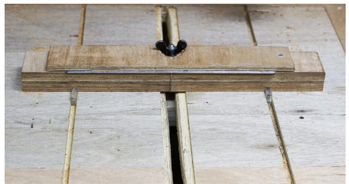
I used the mill to mill a flat surface and two grooves in its bed.
